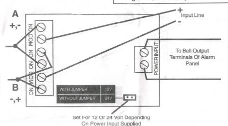
Voltage Output From Alarm Or Similar Device Causes Contact Points To Phone Line From House Phone To Alarm Transmitter, Preventing Blocking Of Outgoing Alarm Message.
